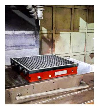
resistance is stronger. Grids can be tapped and punched (diameter 8MM, depth of 20MM or less) for fixing or positioning.
