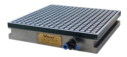
The vacuum chuck is a new clamping tool for non magnetic materials, which use for various machine tools. It can attract any kinds of flat surface work pieces. Weike has two types of vacuum chuck, Grid type needs sealing strip to assist in forming a vacuum area. The multi holes type is an upgraded version of the grid type, which automatically forms the vacuum area, making it more convenient and efficient.
