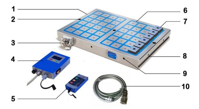
1 Chuck Body 2 Fixing Screw Hole 3 Controller Adaptor 4 Controller 5 Remote Panel (Optional) 6 Epoxy Resin Insulation 7 Padding Block 8 Groove For Clamping 9 Lifting Ring Fixed Hole 10 Cables For Connect Controller, Magnet Body And Power Supply
