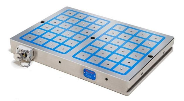
Electro permanent magnetic (EPM) milling chuck is the best magnetic clamping tool at present, which use electro pulse to (de)magnetize. It is safe and reliable when workpiece is clamped by magnetic chuck in mechanical processing." Magnetize and Demagnetize" time is less than 1 second, After magnetization, the magnetic chuck holds the magnetism permanently, and the chuck won't consume any energy at all during the whole machining. It is widely used in CNC machining, milling and die manufacturing.
