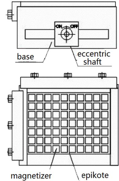
The magnetic chuck has high precision itself; it can guarantee the precision of workpiece from 2um/100mm. As it doesn't need electricity, the workpiece won't move in no power supply condition. And won't generate heat even for long time using.
