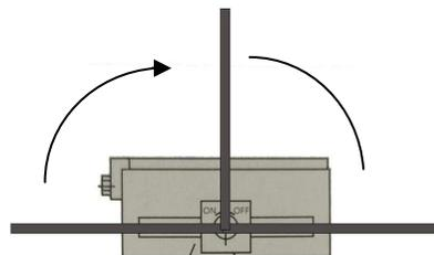
wrench (one of accessories) to rotate the eccentric shaft from “off” to “on” in anti-clockwise direction ( about  $180^\circ$  ). The work piece will be attracted and held in the chuck, see right picture.
